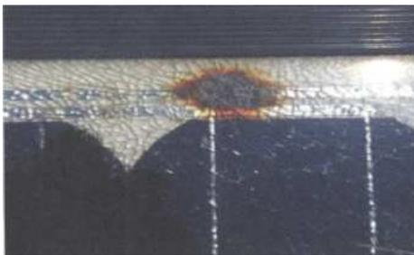
**Figure 2. Example of fire hazard from damaged bus bar.**
