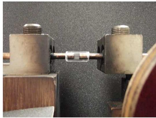
Figure 4. Laboratory arc generator.
