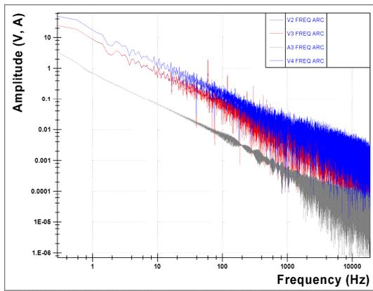
**Figure 6. Spectra of arc fault waveforms shown in Figure 5.**
