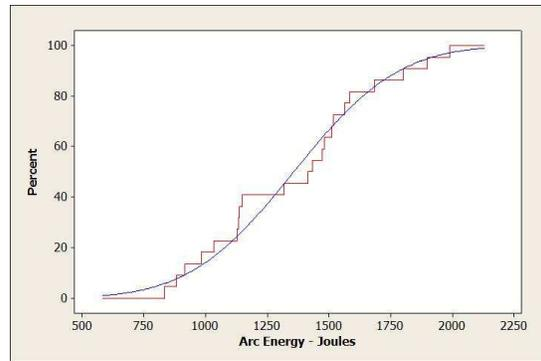
**Figure 7. Cumulative distribution of experimental data where burn through was observed.**
