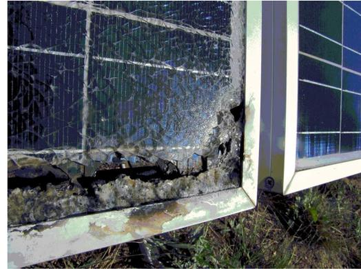
**Figure 3. Arcing to grounded metal frame.**
