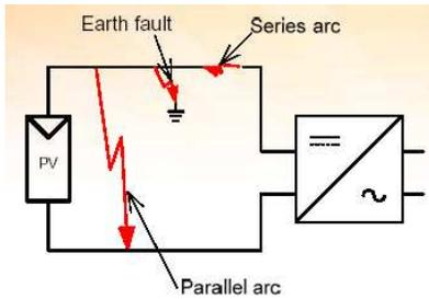
**Figure 1. Series arc fault and parallel arc fault in PV systems.**
